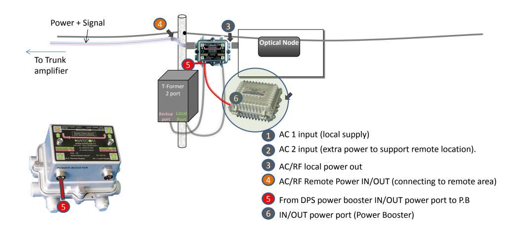
Safecom's patented add-on Power Booster enables to utilize the DPS remote backup technology for longer distance by compensate the voltage drop along the coax or electric cables.
